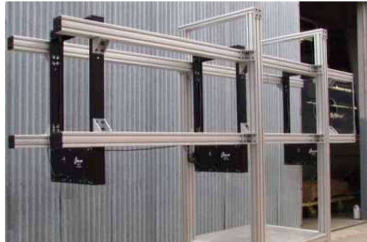
Speed 'Trap' to Measure Projectile Velocity
