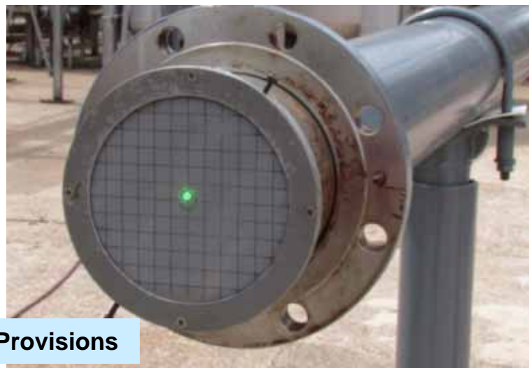
Speed 'Trap' to Measure Projectile Velocity
