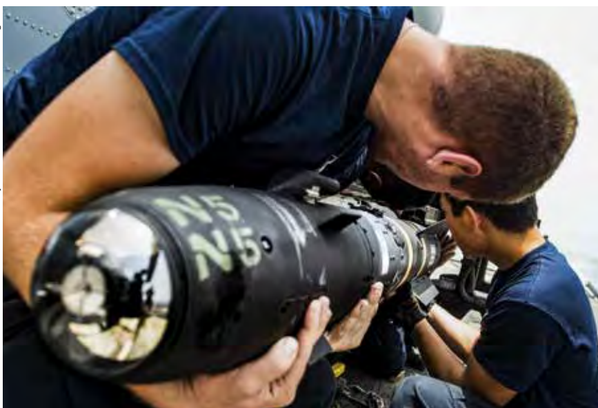
The AGM-114N HELLFIRE metal augmented charge (MAC) variant, i.e. thermobaric, is in use with British forces, which call it an enhanced blast weapon. Pictured: US sailors load an AGM-114 HELLFIRE missile onto an MH-60R SEAHAWK helicopter.
