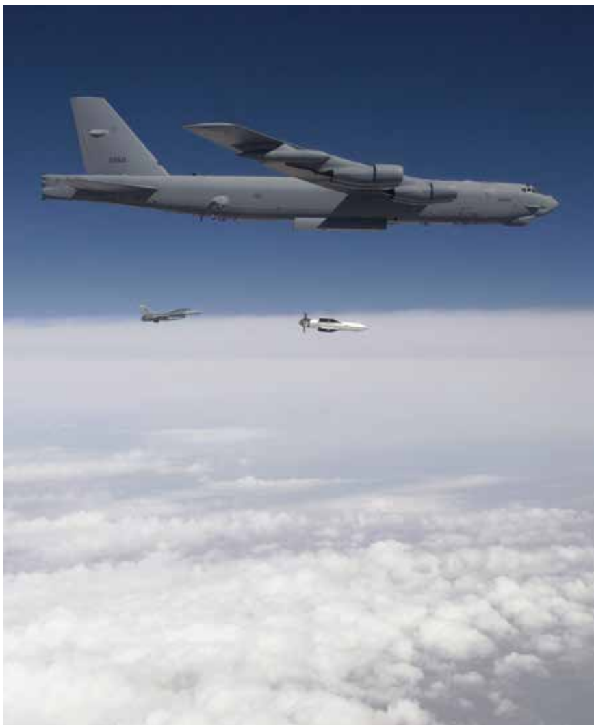
A B-52 releases a test version of the Massive Ordnance Penetrator (MOP) over White Sands Missile Range, N.M. in 2009. The 14,000 kg heavy, 6.2 metre long bomb can penetrate to a depth of 61 metres to destroy command centres and other hardened targets.
