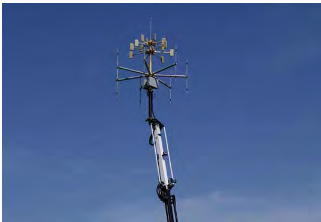
The mast-mounted antenna array of an Airbus Defence and Space passive radar system.
