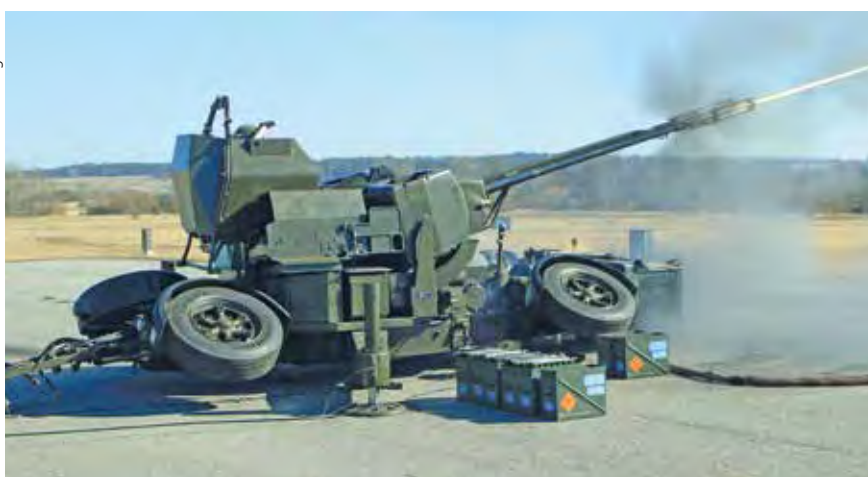
Austrian GBAD-officers agree that with those 1980s Oerlikon-Contraves (now Rheinmetall-Air Defence) 35mm twin guns, they can only fight aircraft- and helicopter-like targets up to 3000m in elevation and 5000m in distance. But in countering UAVs there could be a 2 nd life...
