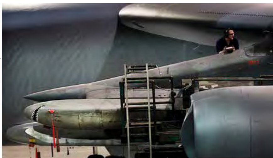
Loading an AGM-86B air-cruise launch trainer missile onto a B-52H STRATOFORTRESS underwing pylon at Minot Air Force Base, N.D.
