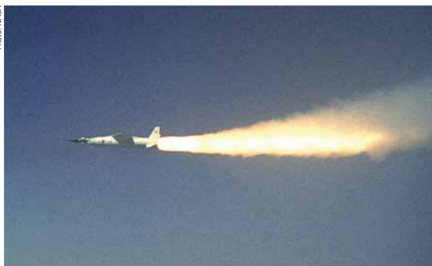
A PEGASUS solid-propellant rocket booster was used to accelerate this NASA X-43A scramjet-powered UAV during a test flight in March 2004.
