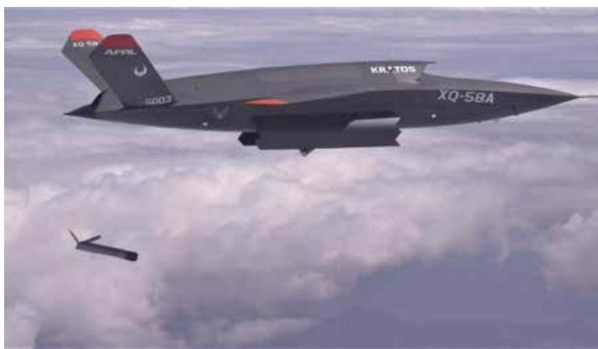
A QX-58A VALKYRIE test aircraft performs the first release of an internally carried smaller UAV.
