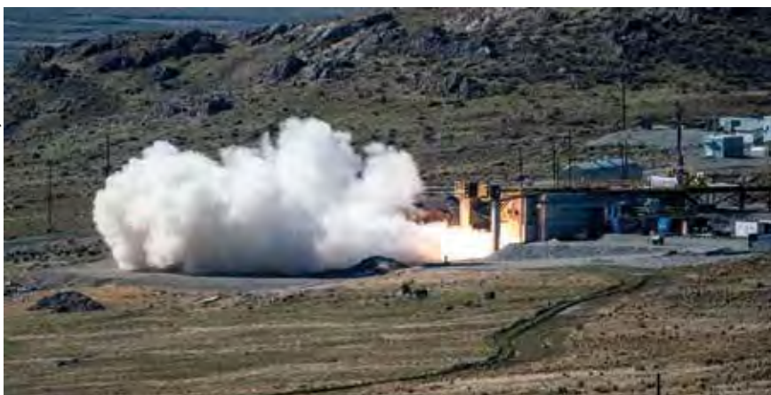
This test firing confirmed the performance of the solid-propellant rocket motor that will be used by the US Navy's Conventional Prompt Strike (CPS) and US Army's LONG RANGE HYPERSONIC WEAPON (LRHW) programmes.
