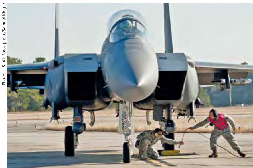
The US Air Force launched flight test activities in 2011 for the F-15E Radar Modernization Program (RMP) to replace the legacy APG-70 mechanically scanned radar with the current AESA-equipped APG-82(V)1.
