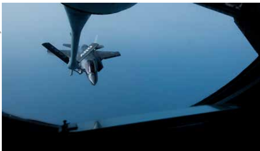
A US Marine Corps F-35B LIGHTNING II receives fuel from the drogue basket attached to the boom of a U.S. Air Force KC-135 STRATOTANKER during an aerial refueling mission near the Horn of Africa, Sept. 15, 2018. The F-35B combines next-generation fighter characteristics of radar-evading stealth, supersonic speed, fighter agility and advanced logistical support with the most powerful and comprehensive integrated sensor package of any fighter aircraft in the U.S. inventory.
