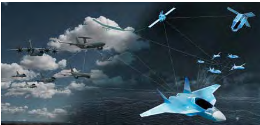
At the heart of FCAS, manned New Generation Fighters teaming with unmanned Remote Carriers as force multipliers will form the Next Generation Weapon System (NGWS).
