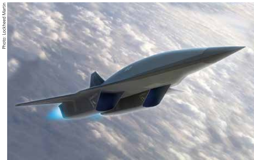
In 2013, Lockheed Martin showed this concept for a hypersonic UAV. Often referred to as the SR-72, this would have been powered by turbine-based combined cycle (TBCC) powerplants in which a turbine engine would have been used at low speeds and a scramjet engine at high speeds. These would have had separate airflow paths, but share a common inlet and nozzle.
