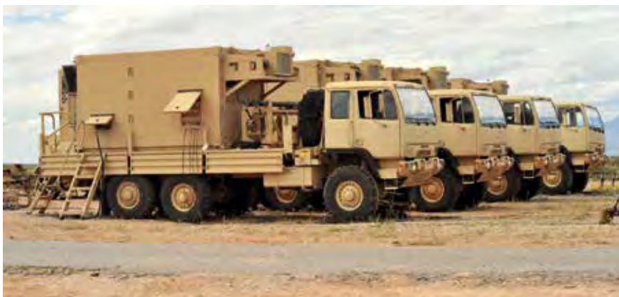
Components of a THAAD Fire Control and Communications (TFCC) System - Two Tactical Operations Stations (TOS) and two Launch Control Stations (LCS)
