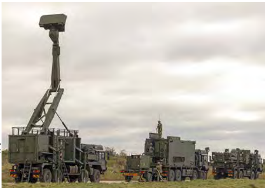
The three elements of the British SKY SABRE air defence system grouped together; the Rafael SAMOC C2 system, the Saab GIRAFFE AMB radar and the CAMM missile system. Britain is now looking for a full GBAD system combining multiple sensors and effectors to deal with broad spectrum threats.
