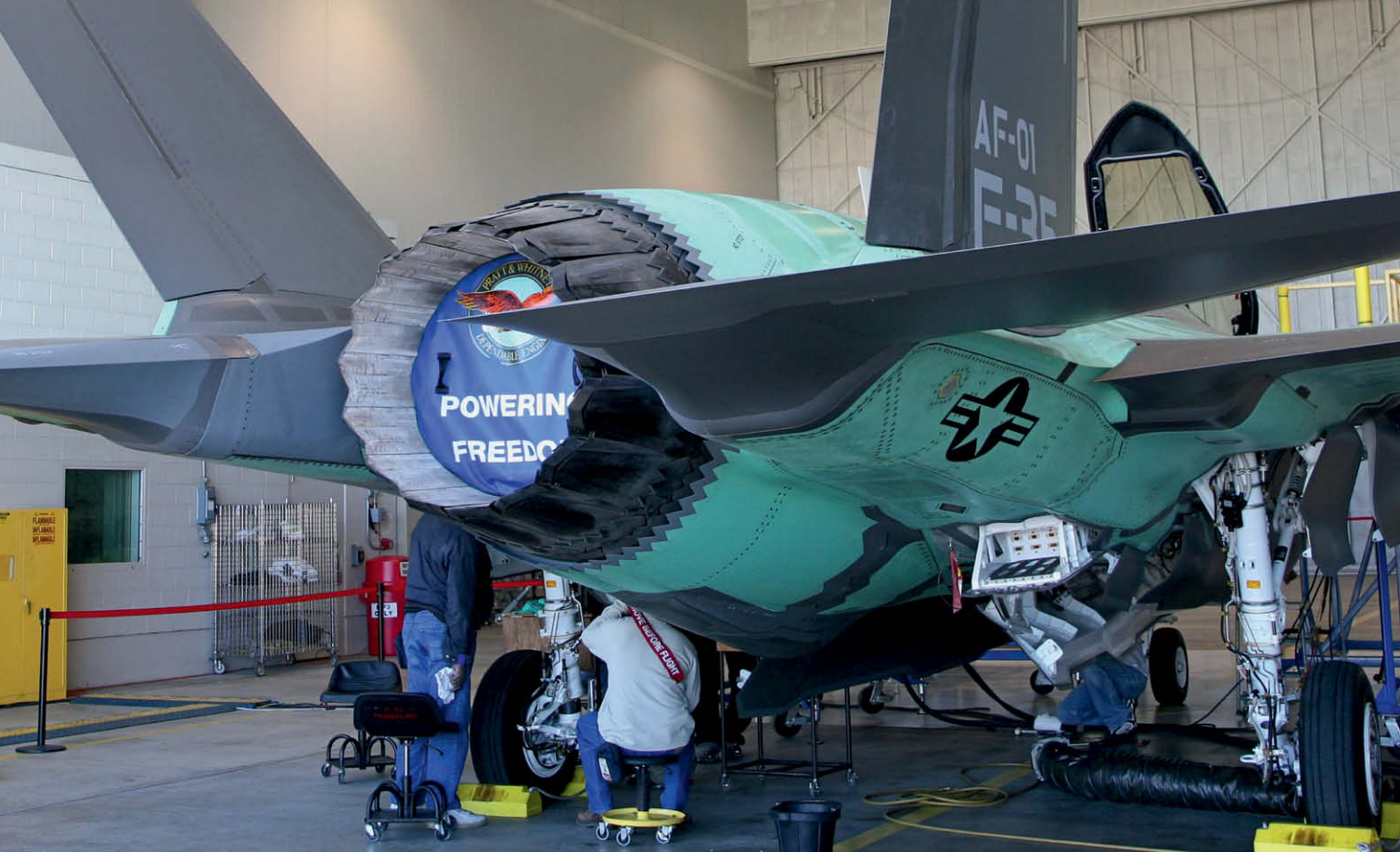
ABOVE: The F135 augmentor or afterburner system has ceramic matrix composites in the exhaust nozzle. PAUL RIDGWAY
