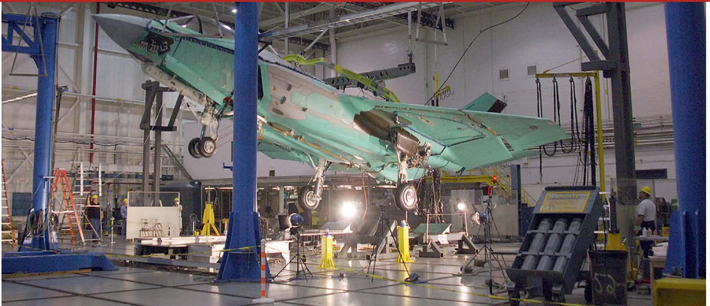
An F-35 CV aircraft undergoing landing gear extension and retraction testing at Fort Worth. GOODRICH
