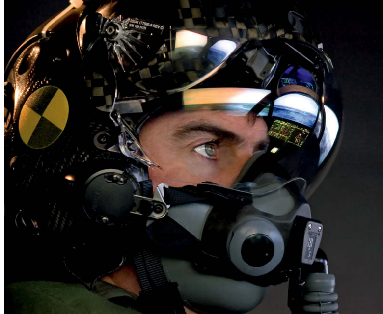
ABOVE: Weighing less than 4 ½ lb (2kg) including the oxygen mask, the HMD comprises the flight helmet and display unit. LOCKHEED MARTIN
