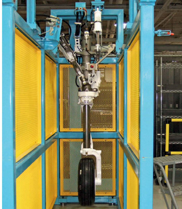
An F-35A CTOL nose gear in a test jig. GOODRICH
