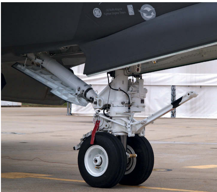
ABOVE: The CV nose gear staged shock strut carries a very complex mechanism to position the launch bar on to the catapult. KEY — MARK AYTON
