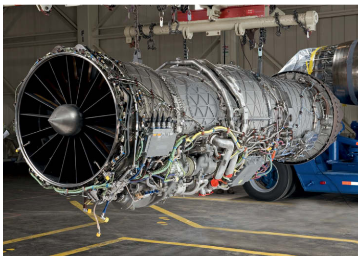
LEFT: This shot shows the F135's first fan stage blisk comprising a solid titanium hub and hollow blades. PRATT & WHITNEY
