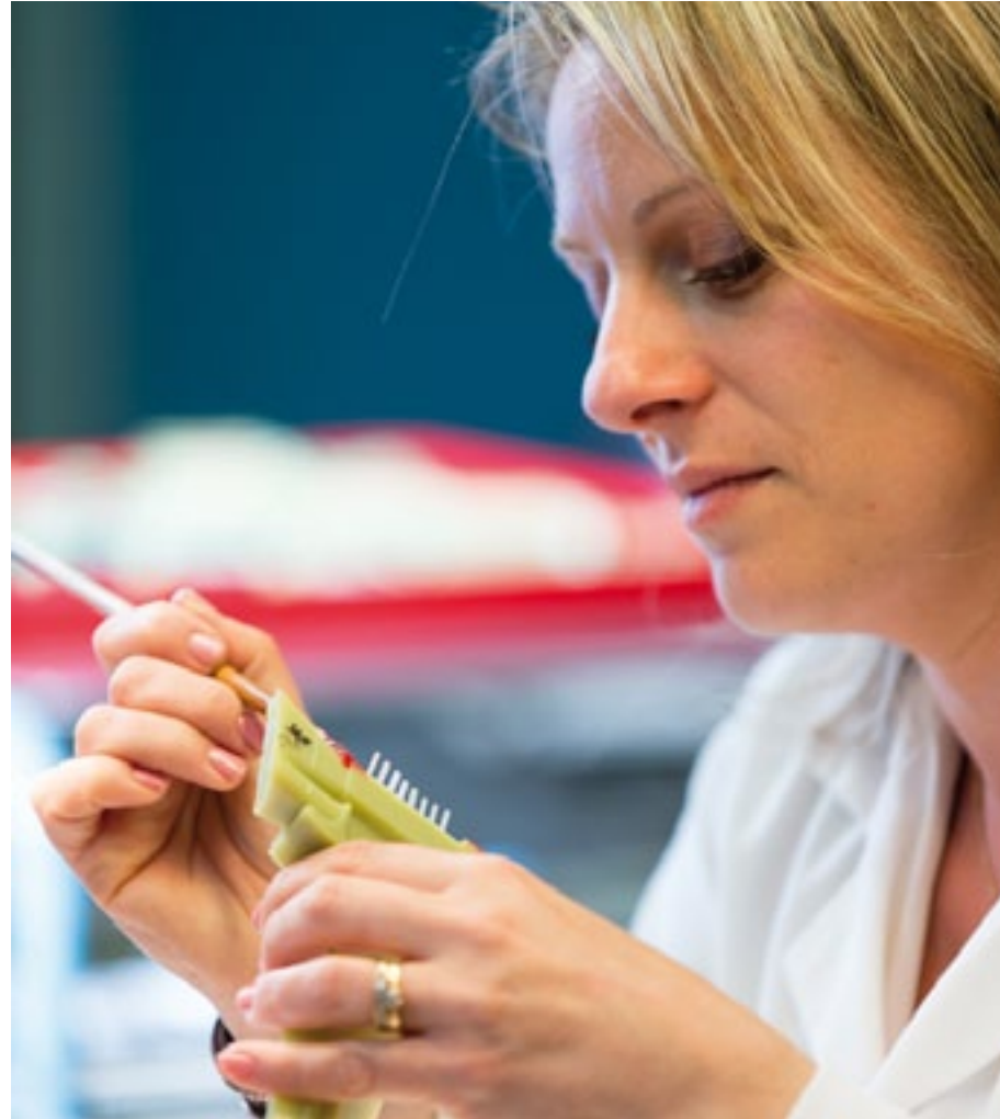
PREPARING LOST-WAX CASTING FOR AN M53 LOW-PRESSURE BLADE
