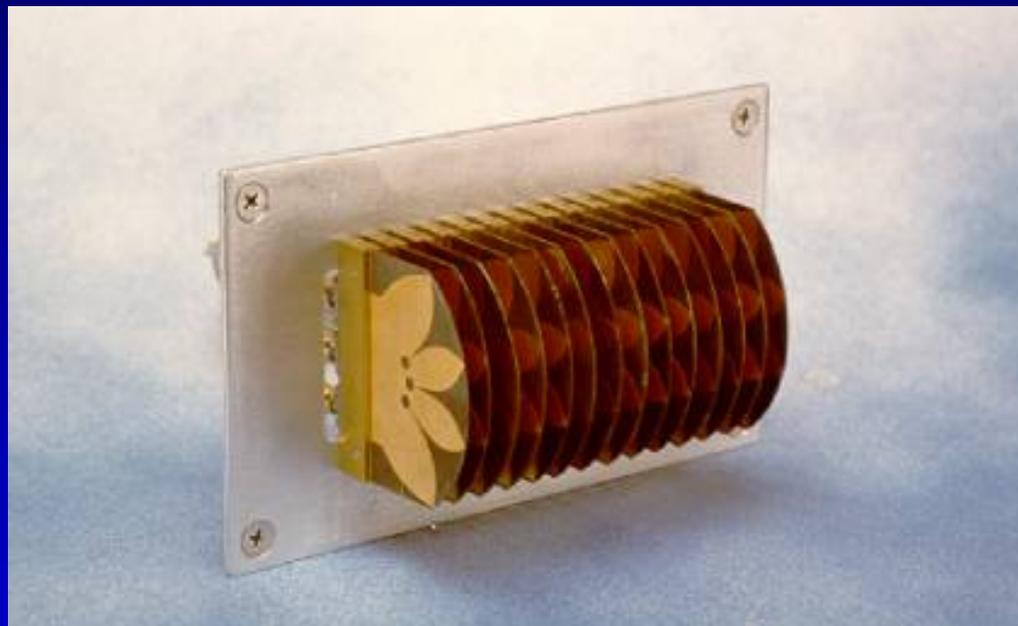
One of the various experimental antenna arrays made and extensively tested during system development
